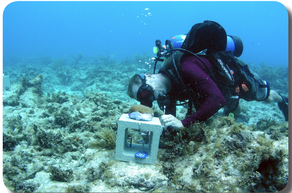
Figure 1. A USGS scientist makes adjustments to a calcification monitoring station at Fowey Rocks Light, off Miami. The research goal is to provide information and datasets that will help us understand cause and effect relationships between environmental variables and coral reef decline.
