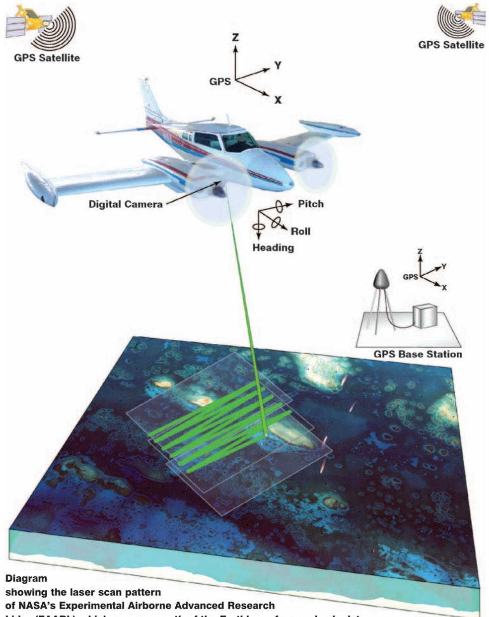
**Diagram showing the laser scan pattern of NASA's Experimental Airborne Advanced Research Lidar (EAARL) which scans a swath of the Earth's surface and calculates ground elevation. Lidar stands for light detecting and ranging [source USGS]**
